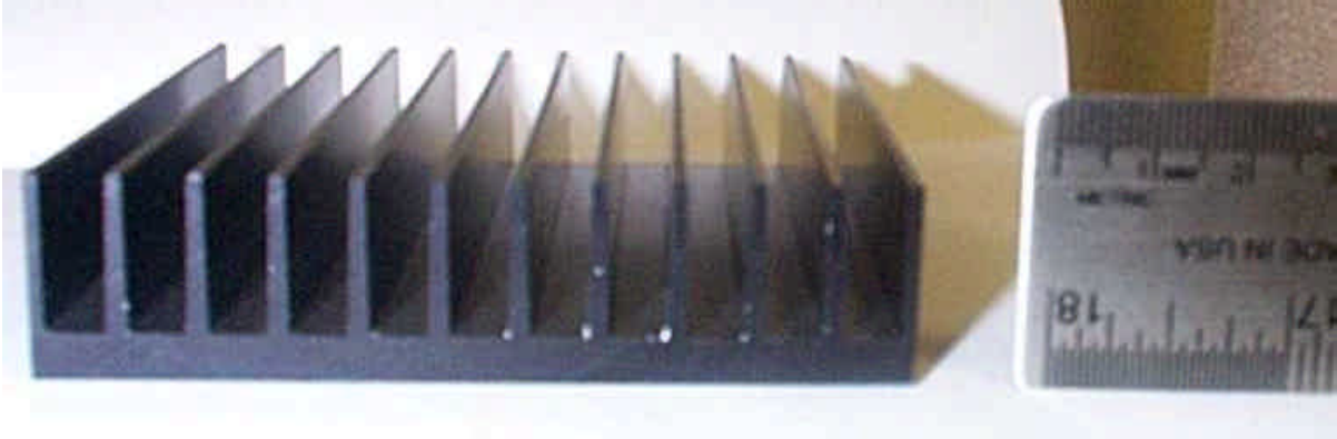
FIG.2c. Large 89mmx76mmx21mm extruded fin heat sink #3.
